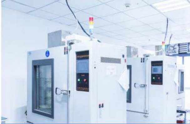
High and low temperature chambers for component aging test
