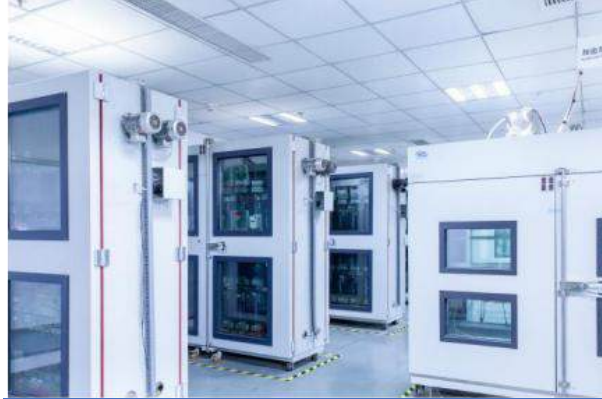
High and low temperature and humidity chambers for accelerated aging tests
